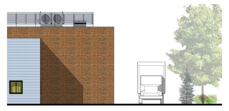
External rooftop mechanical systems may be screened using a parapet or louvers, among other options. Source: KKC
